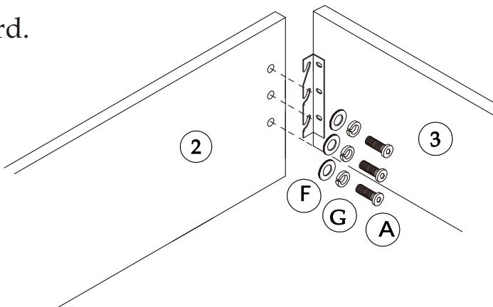
Before tightening the bolts, please ensure the bed frame is square.
